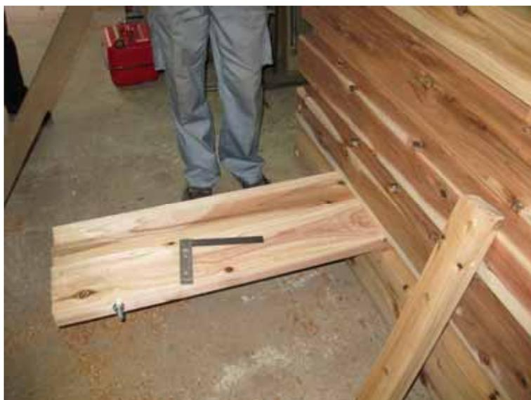
Fig.9-2:杉材積層パネルに階段部固定検討
